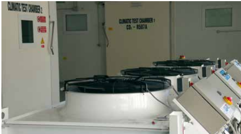
Climatic test chamber for CO 2
