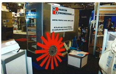
The HASCONWING airfoil profile axial impellers made by HASCON of Italy
