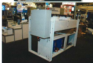
The Concept Plug and Play condenser unit made by Jim Stavris of Rapid Chill with three Maneurop Semi-Hermetic reciprocating compressors
